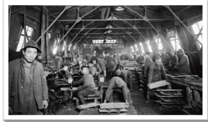
Members of the Chinese Labour Corps rivet together sections of tank in a workshop on the Western Front
